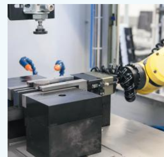
Sample loading and unloading by the ARL SMS-2300 system robot
