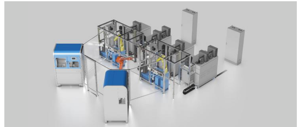
ARL SMS-3300 systems with multiple XRF or OES spectrometers and minimal footprint can be connected to a central preparation cell (possibly supplied by local providers)
