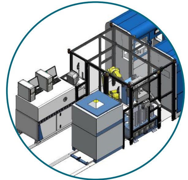
Dual OE-XRF instrument configuration with HS-F1000 preparation machine
