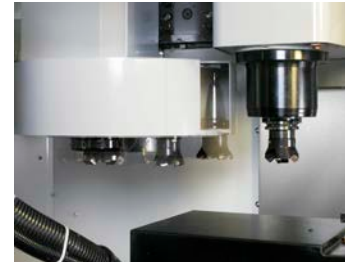
Mini Mill magazine with up to 10 milling heads with automatic milling head change in 5 seconds
