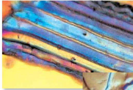
Polymer laminate (left) and scratched sample surface under DIC (right)
