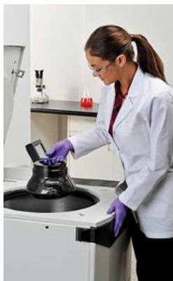
1. Place rotor into the centrifuge chamber
