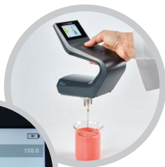
HAAKE Viscotester 3 viscometer as handheld unit
