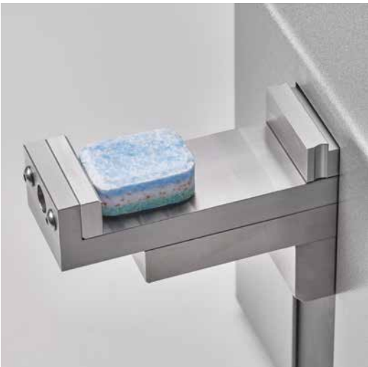
Extended jaw for testing large objects up to 65 mm
