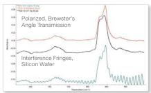
Improve sensitivity and surfaces and suppress interference with polarized measurements.
