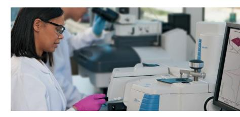
The Nicolet iS50R Spectrometer carries forward all the flexibility and performance of the Thermo Scientific™ Nicolet™ iS50 Spectrometer system, with the added capabilities for the research spectroscopist. The Nicolet iS50R includes dual sources and triple detector optics, multiple on-board digitizers and easy access to spectrometer data and control signals.
