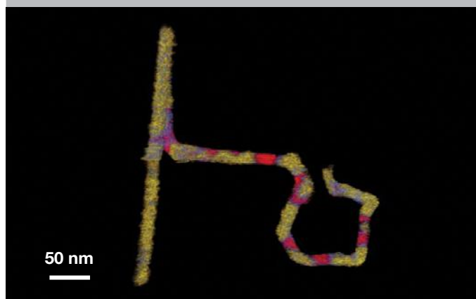
3D EDS tomogram of P-Zn-In nanotubes. Sample Courtesy of Dr. Reza Shahbazian Yassar, Michigan Tech University.
