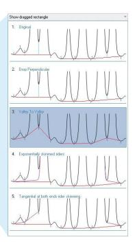
SmartPeaks alternative integration approaches and automatically adds parameters to the processing method for the chosen approach.
