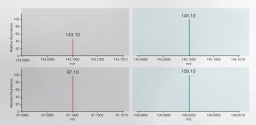
From top to bottom: Estrone, greater relative abundance quantifier ion and lesser relative abundance confirming ion. Testosterone, quantifier ion and confirming ion.
