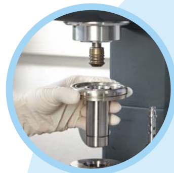
Quick bayonet mountings for short pre- and post-handling time per measurement
