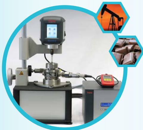
Configuration for pressure cell
