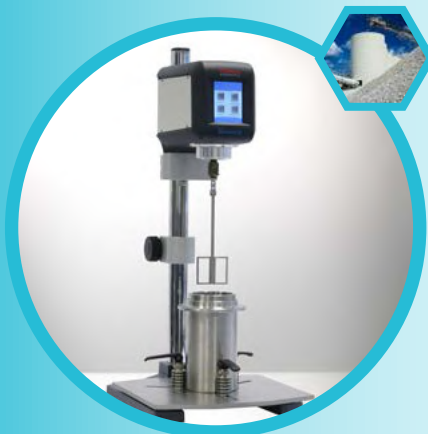
Stand setup with cell for building materials
