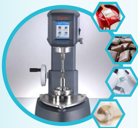
Stand setup with vane rotor
