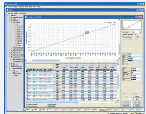
MVR Calibration curve showing real concentrations vs. intensities
