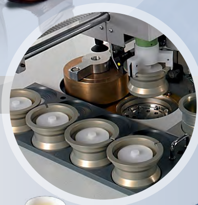
Special cassettes for liquid cell loading
