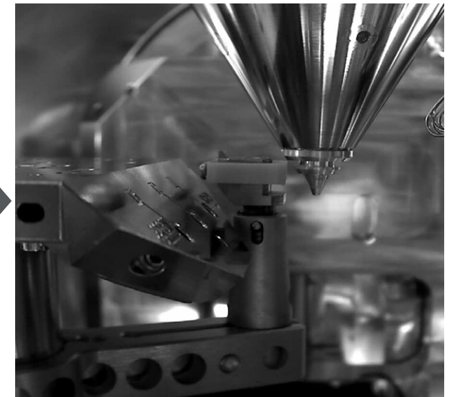
As soon as the PLA is mounted, the stage moves aside and the system is ready for low vacuum imaging up to 500 Pa chamber pressure.
