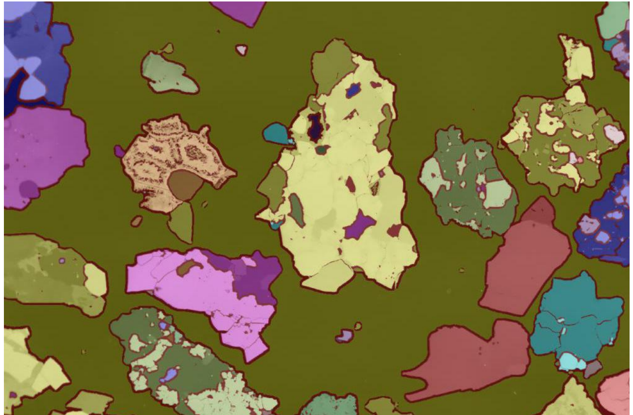
Feature-based image segmentation of a geological sample.
