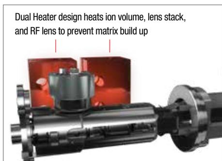
The AEI source is also heated throughout, with RF pre-filter lenses to prevent ion-burn effect into the quadrupole. In addition, the AEI source benefits from an innate ultra-robustness due to a more tightly focused ion beam, which limits matrix burn in the ion path. With the AEI source the maintenance interventions are reduced further, for extended uptime.
