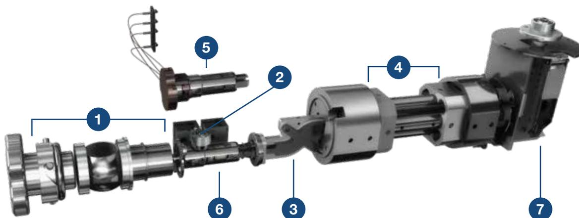
**Ion sources and probes are removable without requiring a break in the vacuum, and they enable you to perform MS and MS/MS experiments on solids in real time while effortlessly switching between electron ionization (EI) and chemical ionization (CI).**
