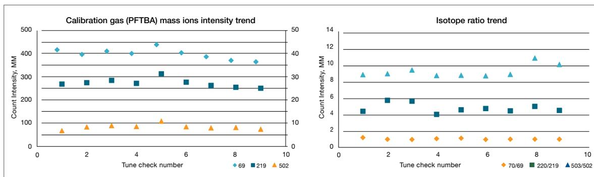
System stability over 400 matrix (QuEChERS food extract) injections without ion source maintenance. The plots are showing the Calibration gas mass ions stability (intensity and ion ratio) over the matrix injection series.
