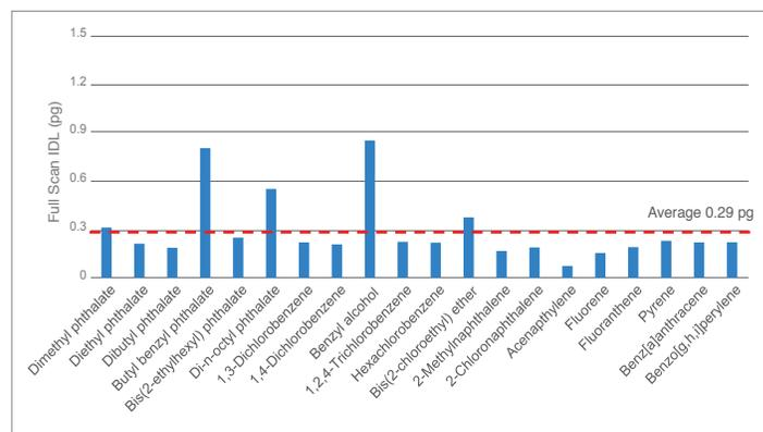
IDL for semivolatiles consistently at sub-ppb levels in full scan acquisition in the range 50-550 atomic mass unit (amu)
