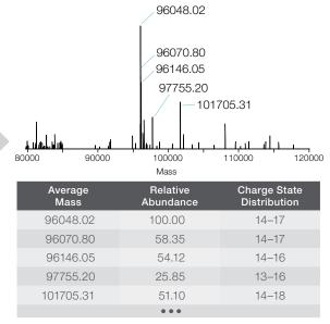
After deconvolution of the PTCR spectrum shown (ReSpect<sup>™</sup> algorithm), several glycoforms of Cytokine Fc-fusion protein were identified. PTCR analysis of the entire native charge state envelope (m/z 4,000–7,000) resulted in the identification of >30 distinct glycoforms of this protein (data not shown).
