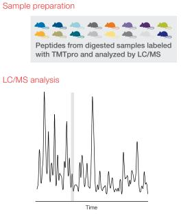
Base peak extracted ion chromatogram of the multiplexed TMT sample. The shaded region highlights a selected MS spectrum.
