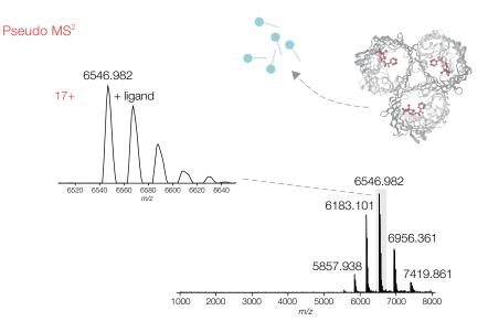
The intact membrane protein-ligand assembly is released from the detergent micelle using source-CID (pseudo MS<sup>2</sup>) and detected in the Orbitrap mass analyzer. The 17+ parent ion with associated ligands is isolated (gray bar) for the next MS<sup>n</sup> step.
