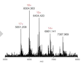
PTCR dispersed the selected ion population to a higher *m/z* range, revealing individual molecular ion species at lower charge states. The interpretation of this spectrum provided accurate information about the mixture of different proteoforms, which were undecipherable in the original spectrum.
