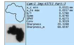
Irregular particles are reliably detected
