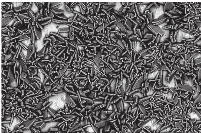
SEM image of Zinc-Phosphate on sheet metal
