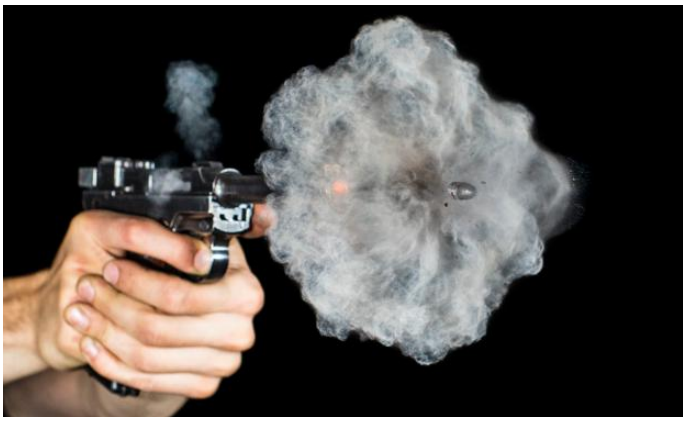
GSR particles are carried in the cloud of smoke after a gun discharge and deposited on the shooter's hand and surroundings.
