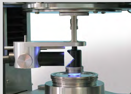
UV curing cell
