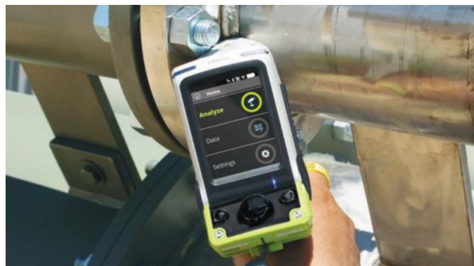
The Niton XL5 Plus in use, analyzing a tight weld in an oil refinery.
