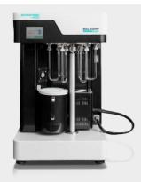
The specific surface area is one of several important characteristics for the evaluation of powder material. This instrument quickly and reliably measures the BET surface area of up to six samples. Measurement and pretreatment are carried out simultaneously. The BELSORP MR 6 is used not only for research applications but also in quality control.
