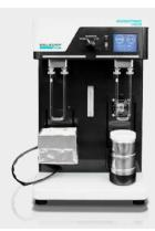
The BELSORP MR 1 is designed for rapid and convenient BET single-point measurement.
