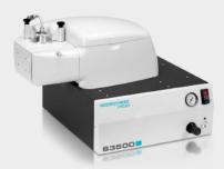
The Microtrac S3500 is a industry-preferred Laser Diffraction (LD) analyzer, ideally suited for various particle characterization tasks. It is the first particle size analyzer that uses three precisely placed red laser diodes to accurately characterize particles like never before.
