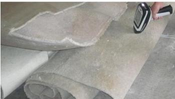
The microPHAZIR $^{\rm m}$  PC analyzer allows users to quickly sort through and identify carpet fibers in a matter of seconds.
