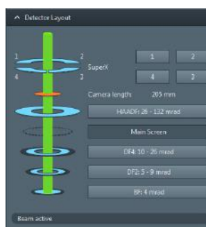
Velox' live optics and detector layout.
