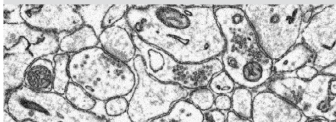
Mouse brain sample. Data acquired by physical slicing at HiVac mode. Imaged in BSE mode at 2 kV accelerating voltage, 0.1 nA beam current, 2 \mu s dwell time. Acquired pixel size 4 x 4 nm. Fine features as vesicles and synaptic clefts can be observed. With permission from Dr. Gabor Nyiri, Institute of Experimental Medicine, Budapest, Hungary.
