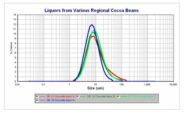
Liquors can also be successfully measured using Isopar G. As shown above, chocolate liquors from several different global regions have different particle size distributions reflecting the different cultural desires in chocolate products.
