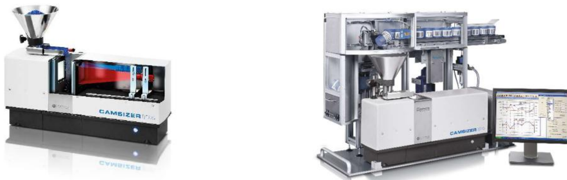
Fig. 1: The CAMSIZER P4 dynamic image analyzer (left). The CAMSIZER P4 can optionally be equipped with an AutoSampler. This allows the fully automatic measurement of up to 12 samples consecutively (right).
