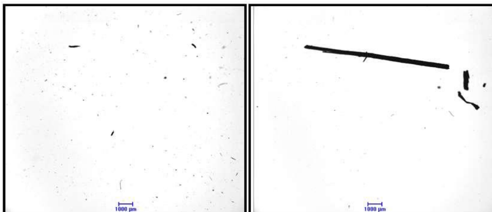
Fig. 4: Typical images recorded by the BASIC camera of the CAMSIZER X2. The scale is 1 mm. Even the largest fibres of the sample, which are up to 10 mm long, can be analysed precisely with the X-Jet module.
