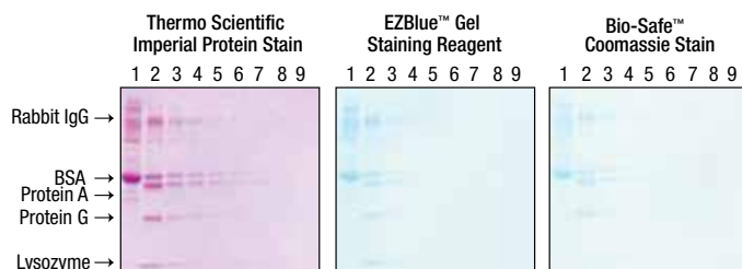
Figure 3. Thermo Scientific Imperial Protein Stain is fast and sensitive. Proteins were separated on 4-20% Tris-glycine gels, stained for 5 minutes and destained 3 x 5 minutes in water. Lane 1: BSA only (6µg), Lanes 2-9: Indicated proteins loaded left to right at 1000ng, 200ng, 100ng, 50ng, 25ng, 12ng, 6ng and 3ng, respectively.
