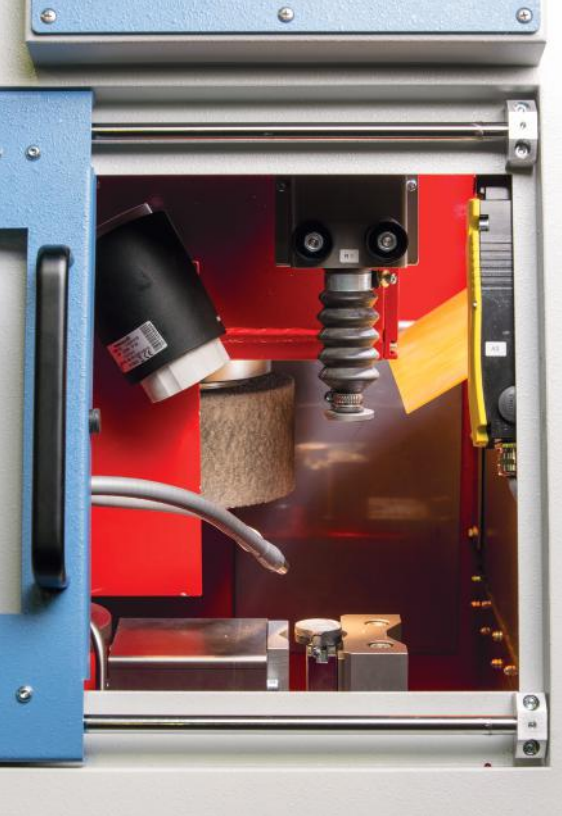
HTS 2000 with hydropneumatic clamping device
