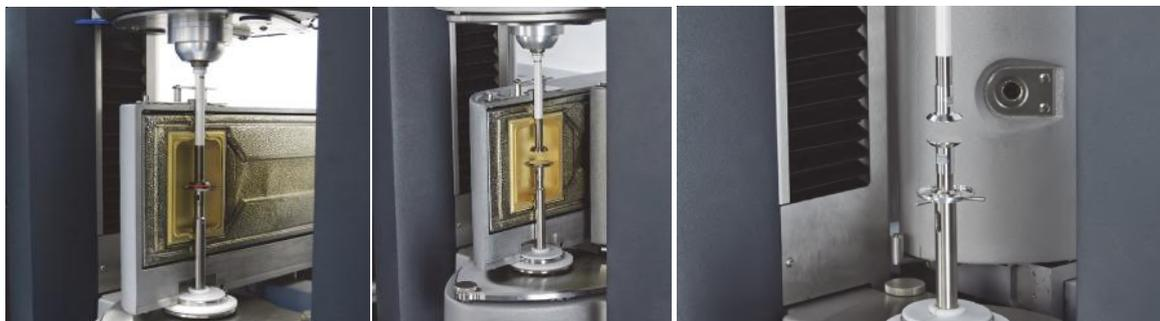
Fig.3: HAAKE MARS with Controlled Tests Chamber (CTC) half-open (left); Standard measuring geometry for CTC consisting of lower shaft with exchangeable plate and upper rotor with ceramic shaft (middle); Disposable measuring geometry for CTC with collection device to prevent chamber fouling (right).
