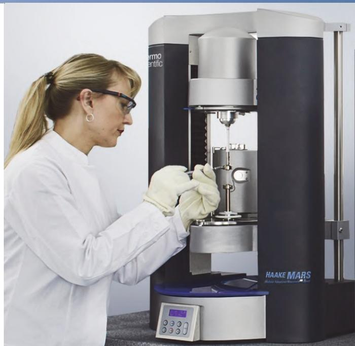
Fig.1: HAAKE MARS with Controlled Test Chamber (CTC).
