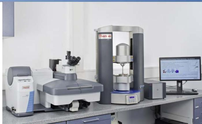
Fig.1: Combination of a HAAKE MARS rheometer with RheoRaman module and adapted Nicolet DXR Raman microscope.
