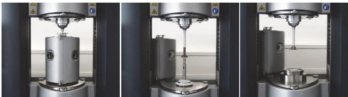
Fig. 2: HAAKE MARS with Controlled Test Chamber (CTC) in measurement position (left); in parking position (middle); in parking position and Peltier temperature control modules for parallel plates and cone & plate mounted (right).
