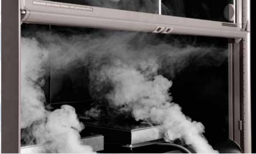
Standard fume cupboard with heating source
