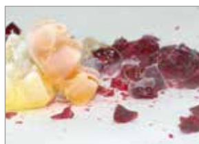
Material embrittled with liquid nitrogen
