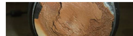
Debris Buildup Around the Detection Section
