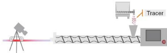
Fig. 2: Residence time distribution measurement set up
