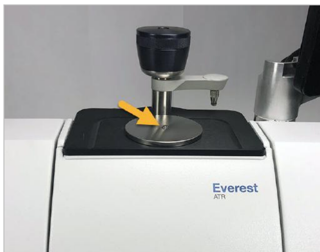
Figure 3-1: Measure a liquid with ATR
