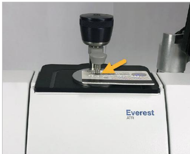
Figure 3-2: Measure a solid with ATR
