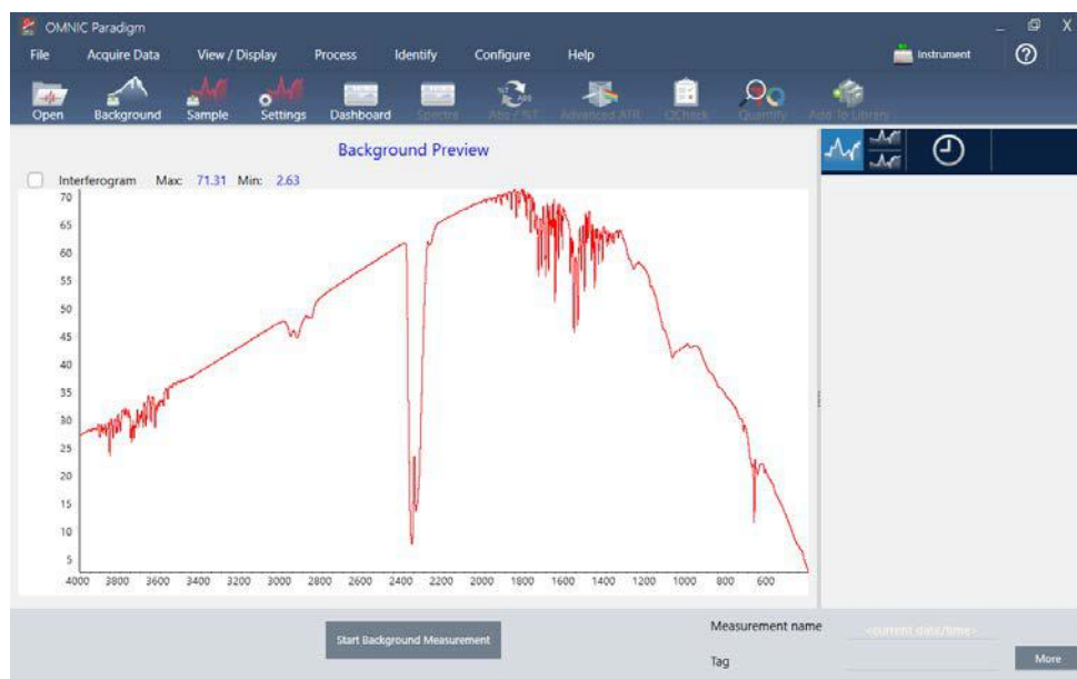
Figure 3-2: Background spectrum from a transmission accessory that has been purged
