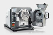
The DM 400 is the new comfort model for fine grinding of medium-hard, hard and brittle materials down to 0.05 mm. This model is based on the well-proven DM 200 but offers improved safety features due to the automatic locking of the collecting vessel and grinding chamber, as well as particularly convenient operation thanks to the motor-driven grinding gap adjustment with digital gap display. The clearly structured display shows all grinding parameters.
