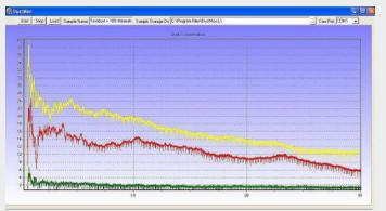
The Y- axis shows the Dust concentration in percent, the X-axis shows the measurement time (typically 30 seconds per measurement) while the graph shows the result of three samples with a different amount of Dust: Very dusty (Yellow) | Less Dust (red) | Dust free (green)
