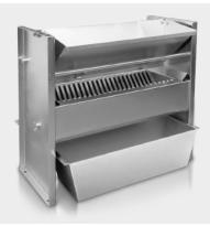
A faultless and comparable analysis is closely linked to an accurate sample handling. Only a sample representative of the initial material can provide meaningful analysis results. Sample splitters ensure the representativeness of a sample and thus the reproducibility of the analysis.
