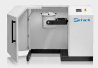
The TM 300 Drum Mill is used for the preparation of granules and powders. The grinding process is performed either in dry or wet conditions. The drum mill can be operated either as a Ball or as a Rod Mill by using the corresponding module. A sufficient number of balls or rods is required for an effective grinding process. Typically, a final fineness below 20 microns is obtained.
