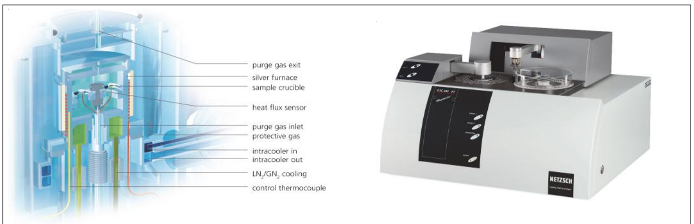
Fig. 8: NETZSCH DSC 204 F1 Phoenix® (right) and cross section through its DSC cell (left).
