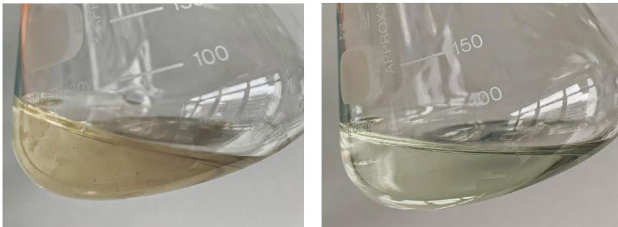
Figure 1. Wastewater samples before (left) and after (right) hot plate digestion procedure
