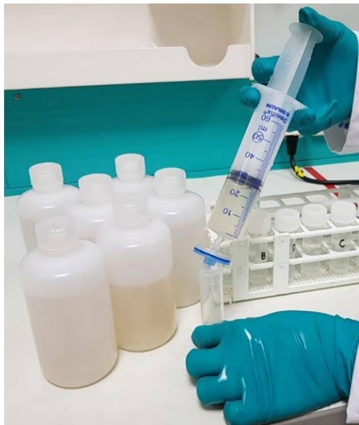
**Figure 5. Collection of river water samples and sample filtration**
