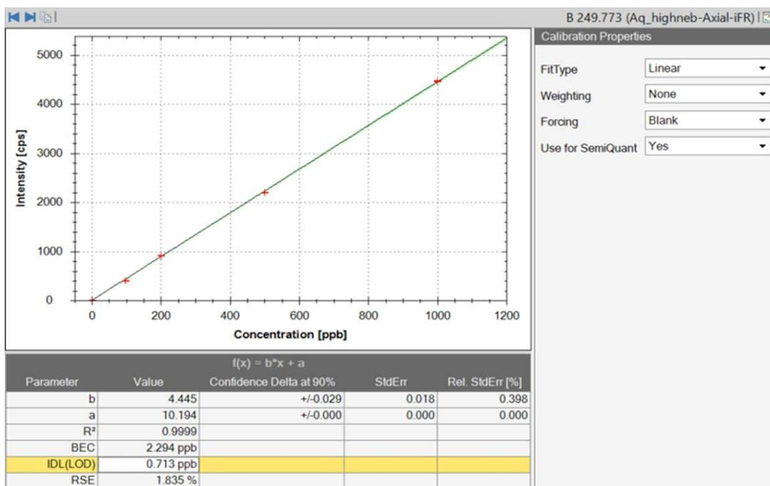
Figure 1. Calibration curve for B 249.773 nm in Axial viewing mode. This is found under the Concentrations section in the Qtegra ISDS Software LabBook and below this plot the limit of detection ( $X_{LD}$  as IDL) is displayed.
