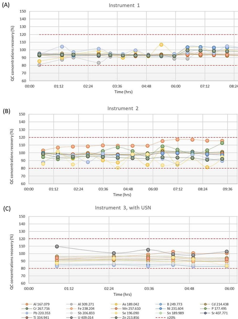
**Figure 4. Long-term experiments demonstrating recoveries of target elements in the QC standard AQO-128-151, 1,000x diluted, data obtained on three distinct iCAP PRO XP ICP-OES Duo systems.** The dashed line represents the maximum allowed recovery interval ( $\pm 20\%$ ) as specified in the DIN EN ISO 11885:2009 method. Additional experiments using the USN (panel C) were run in the customer laboratory where a smaller number of measurements were made.
