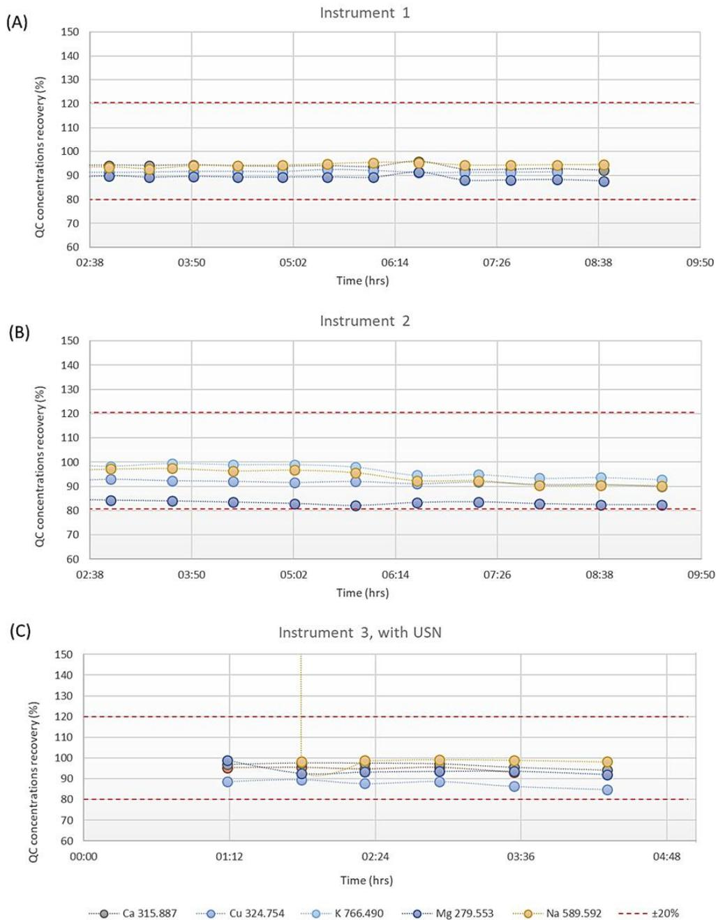
**Figure 5. QC standard recoveries of AQO-127-711, 100x diluted, in stability experiments on three different iCAP PRO XP ICP-OES Duo systems.** The dashed line represents the maximum allowed recovery interval ( $\pm 20\%$ ) as specified in the DIN EN ISO 11885:2009 method. Additional experiments using the USN (panel C) were run in the customer laboratory where a smaller number of measurements were made.
