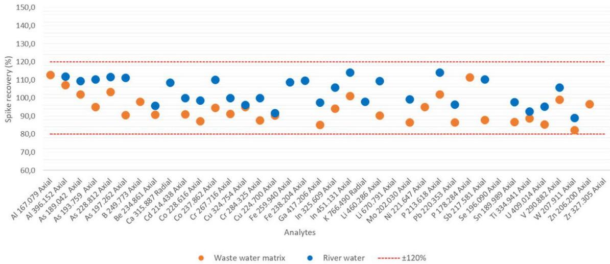
**Figure 2. Spike recoveries in river water sample and laboratory simulated wastewater matrix.** The dashed line represents the maximum allowed recovery interval ( $\pm 20\%$ ) as specified in the DIN EN ISO 11885:2009 method.
