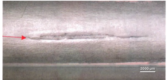
Figure 2. Image of a failed bend test.
