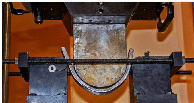
Figure 2. Image of a failed bend test.
