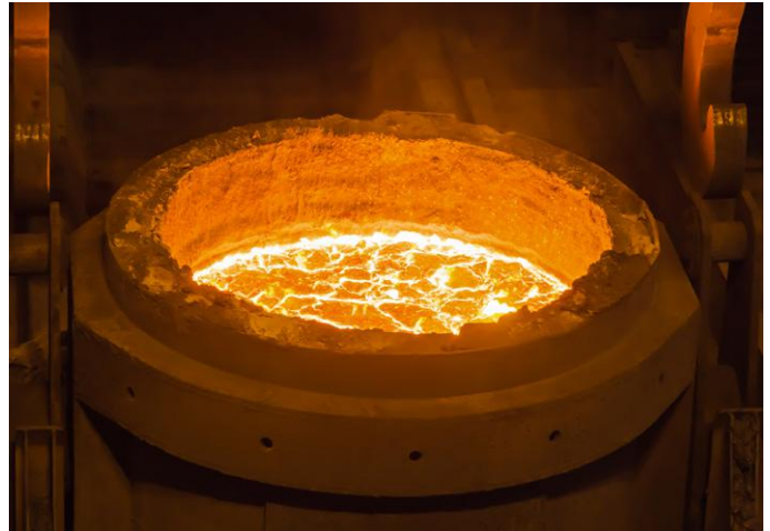
Steel refining is performed in a ladle where deoxidation, desulfurization and inclusion flotation may occur.
