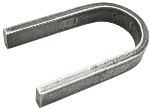
Figure 1. Bend test (top) and tested piece (bottom).
