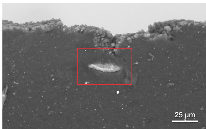
Figure 6. Backscattered electron image showing the position of another type of filler.
