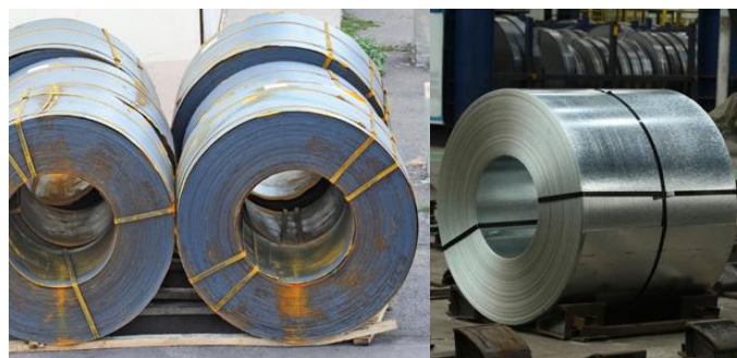
Figure 2. Hot-rolled coils or "black bands" in the left image show black oxide scale formed during reheating and red rust which formed at ambient temperature. The right image shows a hot-rolled steel coil after pickling.
