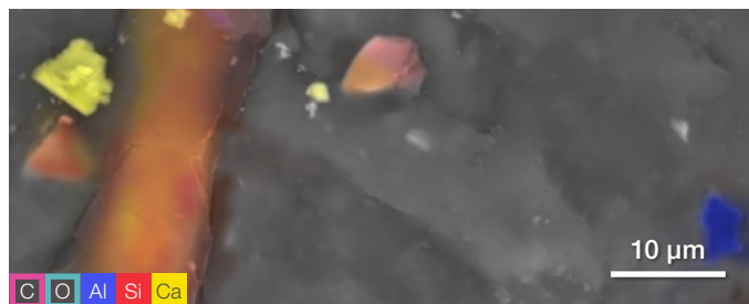
Figure 3. Top: high-mag view of the area presented above in grayscale. Bottom: ChemiSEM image. Only the elements of interest have been selected to highlight features of interest. Dwell time 1 us, total acquisition time 40s.
